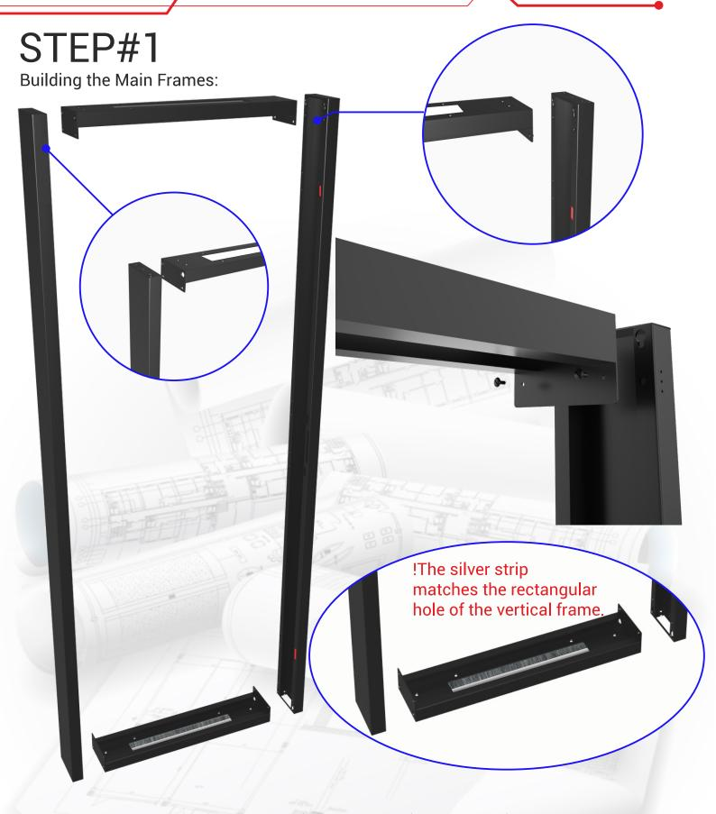
Combine the Horizontal (package 5/5) and Vertical (package 1/5) frame parts into one single frame.
